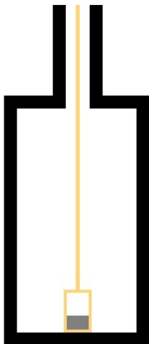
Figure 4: Sketch of the experimental setup. An outer tube of graphite with an inner alumina crucible and tube connected to an argon source. The atmosphere inside the tube was purged with argon before and during the experiments, and argon was blown at different rates through the tube in each experiment.
