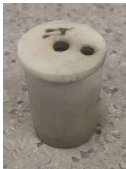
Figure 5: Alumina crucible after finished experiment. The middle hole was used for the alumina tube, while the smaller hole was used as the outlet for the gas and vapor.
