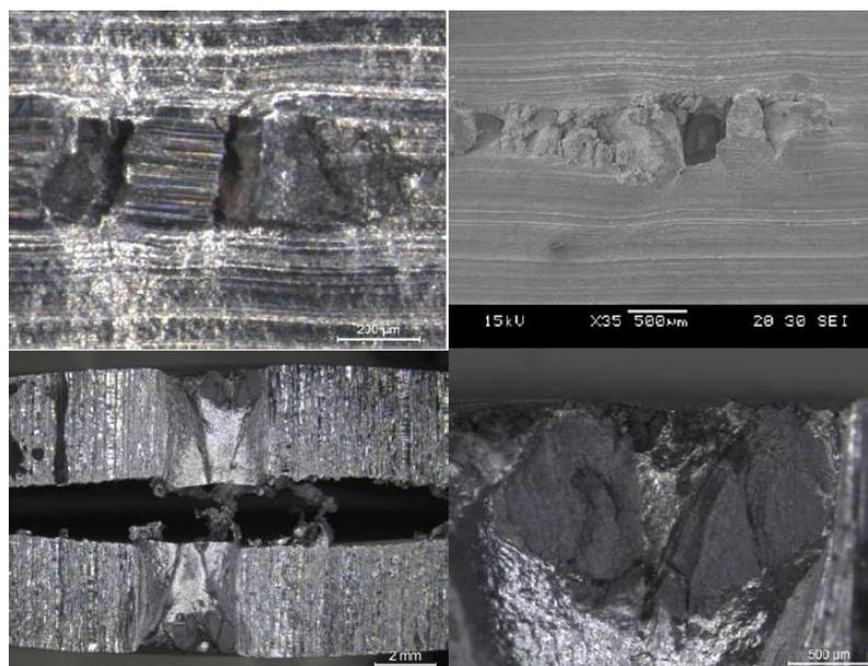
Figure 1. Magnifications of defects created in the extruding process.
