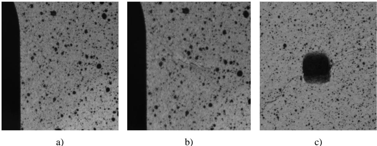
Figure 7. DIC images of a sample before (a) and after (b) crack initiation in the proximity of the fillet radius. Cracks developing from the notch (c).
