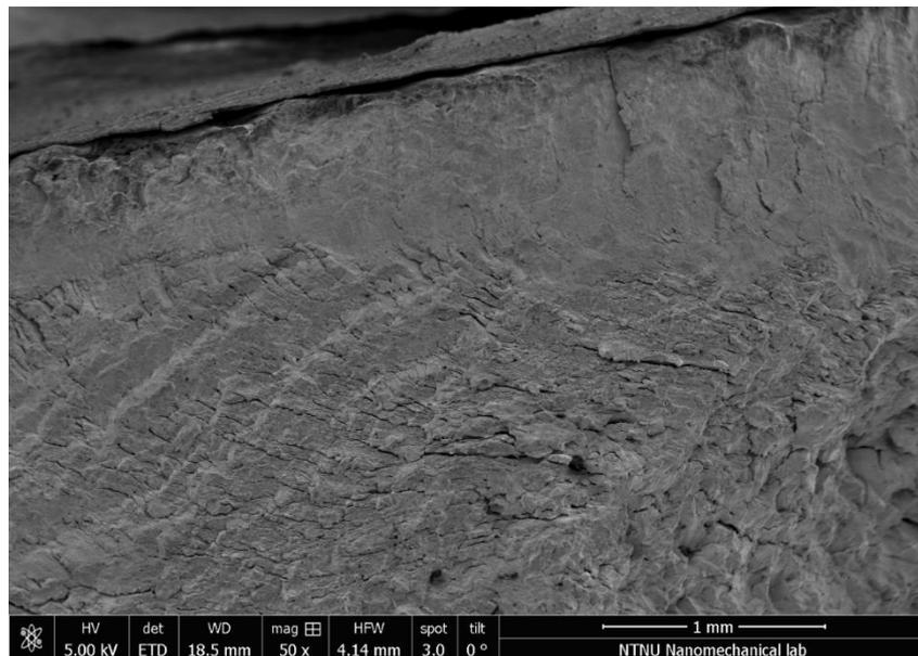
Figure 12. Crack initiation and propagation on a specimen tested at 10 Hz and at a strain range of 0.15 %. On the upper surface, the layer of paint for DIC can be seen.
