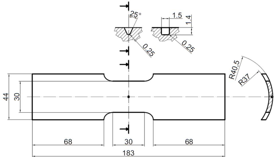
Figure 2. Nominal dimensions of the specimens and of the notch practiced.
