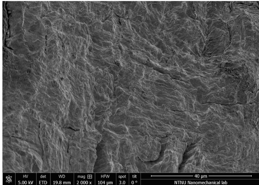
Figure 13. Crack propagation striations on a specimen tested at 10 Hz and at a strain range of 0.15 %. Secondary cracking can be observed.
