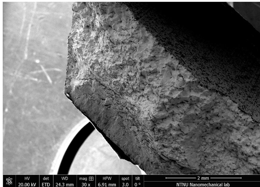
Figure 9. Crack initiation, propagation and plastic fracture on a specimen tested at 5 Hz and at a strain range of 0.15 %.
