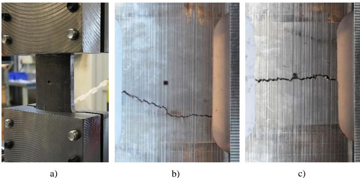
Figure 5. The pictures show the sample in the custom-made, curved clamping system (a), two different crack paths on notched samples (b, c).
