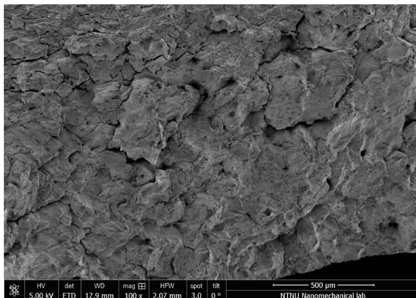
Figure 10. Grain de-cohesion at the final plastic fracture on a specimen tested at 10 Hz and at a strain range of 0.15 %. The fracture location both for the present figure and for the previous fig. 9 is analogous to the one presented in fig. 7b.
