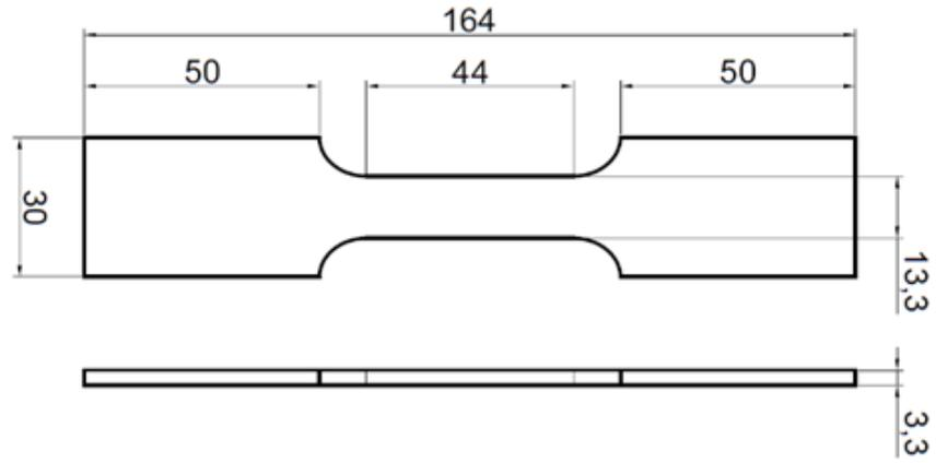
Figure 3. Geometry of the tensile specimens for material calibration.
