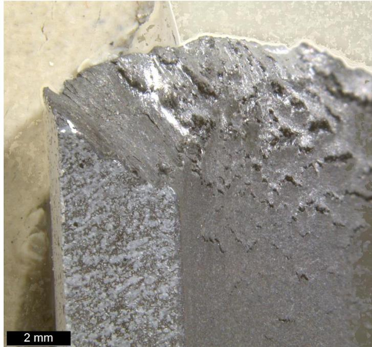
Figure 11. Side view of a failed specimen. The shear crack propagation, the multitude of diffused secondary cracks and the final plastic tearing executed at the end of the test are distinguishable.
