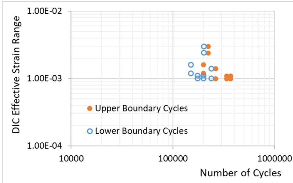
Figure 8. Summary of the strain range detected by DIC in the crack initiation sites. The number of cycles is to crack initiation and the lower and upper boundary cycles are the cycles of the DIC window immediately before and after the crack initiation.
