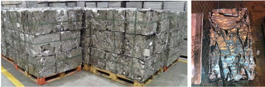
Figure 4 The compacted sheets used in the remelting trials
