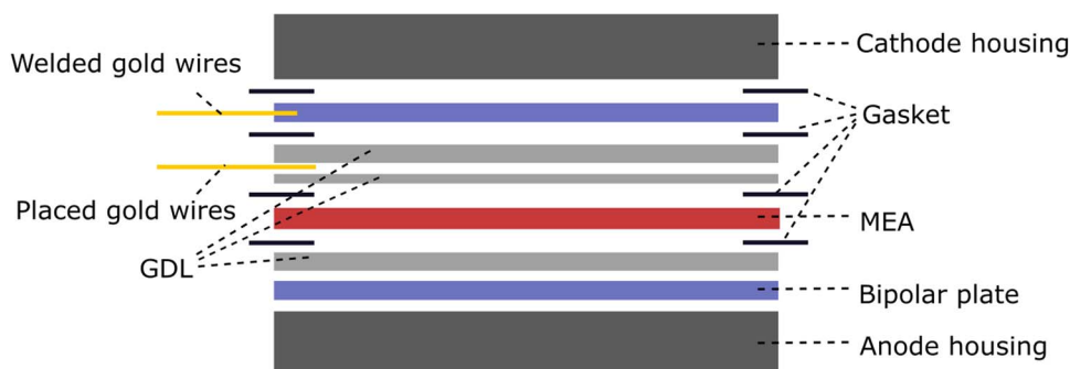
Figure 1. Setup for in situ measurements of ICR as seen from the side with Cathode housing, Gold wires welded to bipolar plate, Gasket (preventing contact between gold wires and other electrically conducting parts of the fuel cell), Gold wires placed in between to sheets of Gas Diffusion layers, Membrane Electrode Assembly, Gas Diffusion Layer, Bipolar plate and Anode housing.
