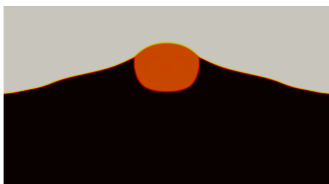
Figure 15: Surface instabilities induced by spurious currents.
