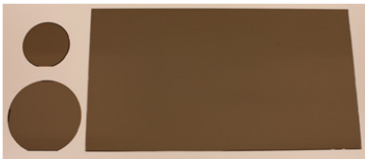
Fig. 4. Photograph showing a Pd-23%Ag film applied on 4" and 6" silicon wafers and a 55 \times 30 cm^2 glass substrate.
