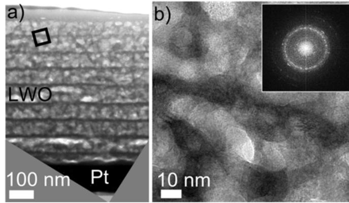
Figure 2. (a) TEM image and (b) high resolution TEM (HRTEM) image of LWO film deposited from citric acid solution, heat-treated at 800 °C for 30 min by RTP. A fast Fourier transform of the HRTEM image is displayed in inset showing a polycrystalline pattern corresponding to LWO without preferential orientation.
