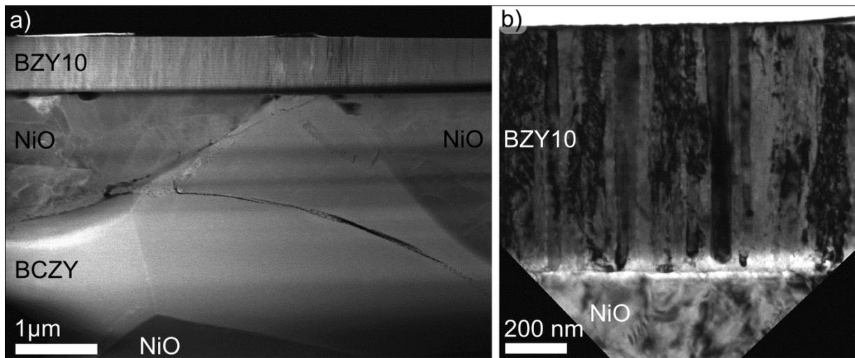
Figure 5. (S)TEM images of BZY film deposited by CSD (20 layers) on a dense BCZY27-NiO anode and annealed at 1000 °C. (a) Overview STEM HAADF image. (b) Higher magnification TEM image of the columnar BZY growth on a NiO part of the anode.
