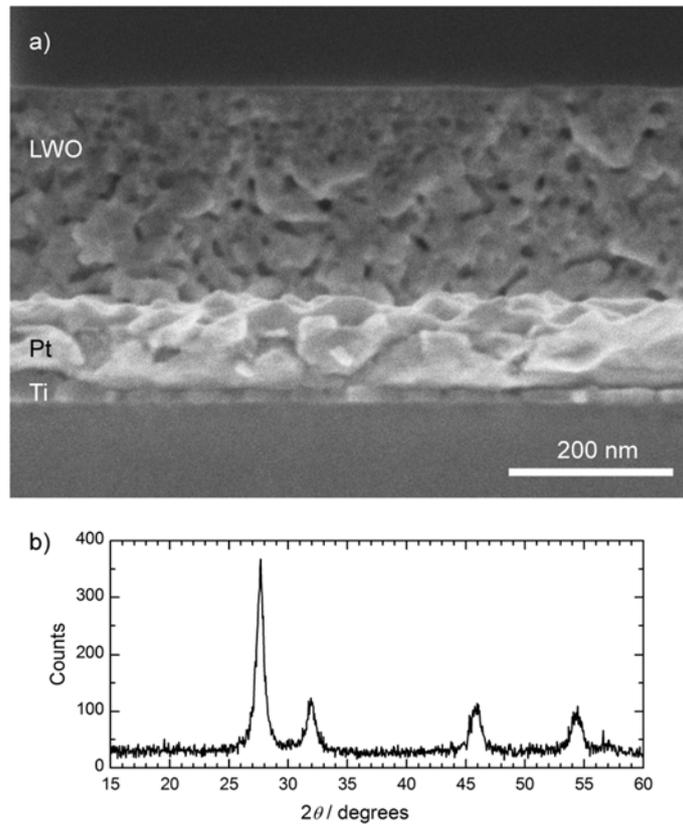
Figure 3. (a) SEM image of LWO thin film deposited from an EDTA-stabilized aqueous solution on platinized Si. 10 layers were deposited with pyrolysis at 500 °C on a hotplate between each layer. The film was finally crystallized at 800 °C for 4 h in air. (b) X-ray diffractogram with grazing incidence  $\theta = 1^\circ$  of the LWO thin film imaged in (a).
