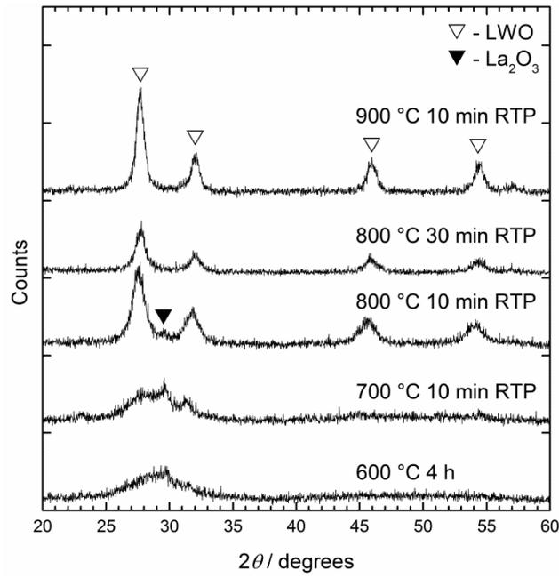
Figure 1. X-ray diffractograms with grazing incidence  $\theta = 1^\circ$  of five LWO thin films deposited from citric acid solution. After the final layer deposition and pyrolysis the films were annealed for crystallization and sintering as indicated.
