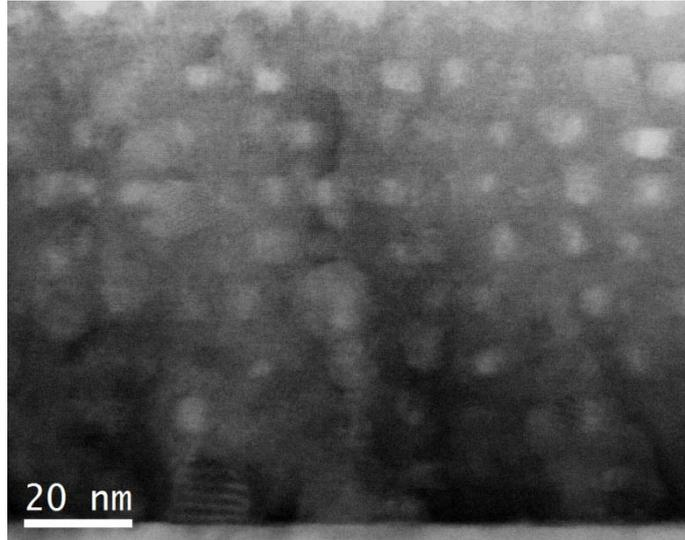
Figure 4. STEM bright field image of an epitaxial BZY film on MgO annealed at 1000 °C. The regular STEM-brighter spots are volumes of lower density (voids), in an otherwise monolithic (single crystal) matrix.
