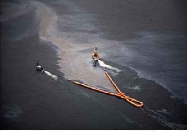
Figure 1: Oil boom operated in calm sea.
