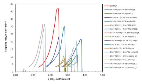
Fig 2. Precipitating system desorption curves at 80°C
