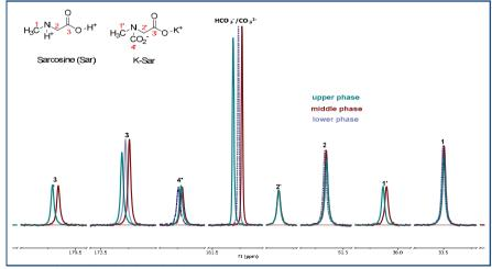
Fig 5 13C NMR spectra of three phases in loaded K-Sarcosine system.
