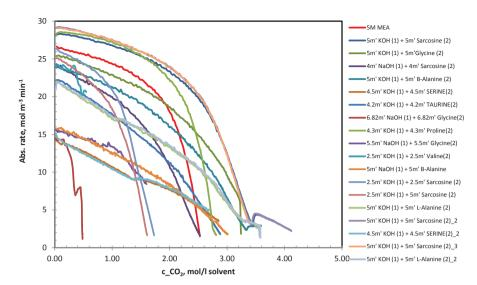
Fig. 1 Precipitating systems absorption curves at 40°C
