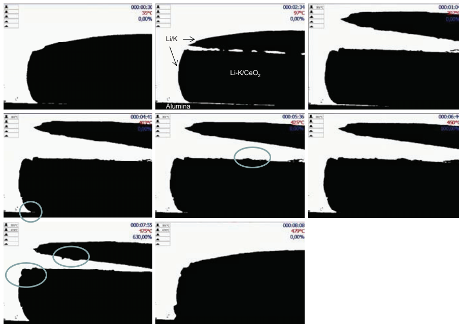
Fig. 7. Pictures taken by optical dilatometer upon annealing in air of Li-K/CeO 2 membranes. Circles highlight changes occurring during annealing. Notice that the excess of Li/K carbonate after dip-coating of the porous disk has delaminated from the surface of the ceramic upon annealing from room temperature to 90 °C
