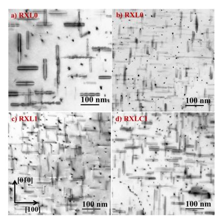
**Fig. 3** TEM bright field images from each of the three Li-containing alloys at near peak hardness condition (4h AA at 195 °C). (a) RXL0, TEM specimen 1, (b) RXL0, TEM specimen 2 (c) RXL1 and (d) RXLC1.All images are taken along the <001>Al zone axis. The double contrast lines in the micrographs are needles along the two [100]Al directions in the viewing plane. The crystal directions are indicated by arrows in (c).
