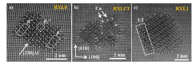
**Fig. 4** Unprocessed HAADF-STEM images from (a) RXL0, the arrow points out a stacking fault along  $a_{\beta^n} \parallel \langle 230 \rangle_{Al}$ . The dashed lines indicate  $\beta$  "and  $\beta_2$ " unit cells, (b) RXLC1, where bright Cu columns can be observed. Two Cu columns are pointed out by arrows. (c) RXL1, the dashed lines indicate a U2 region. The crystal directions, as indicated by arrows in (b), are the same in all three images.
