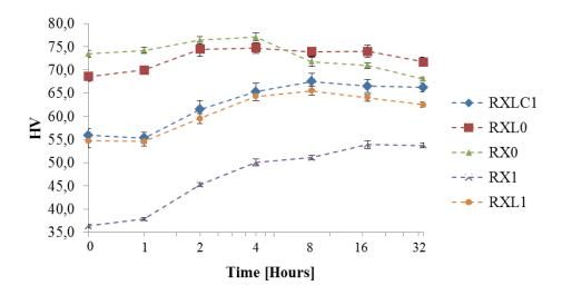
**Fig. 2** Vickers hardness plotted as a function of artificial ageing time at 195 °C. Note that the x-axis has a logarithmic scale. RX0 (top) and RX1 (bottom) signify the dense and lean
