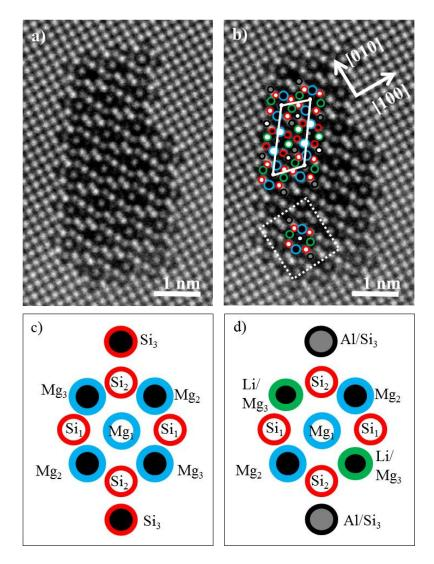
Fig. 5 (a) 'Smart Aligned' image of a  $\beta$ " precipitate cross section in RXL0. (b) Partial atomic overlay on the precipitate in (a), where a unit cell of  $\beta$ " is indicated by a white, solid lin parallelogram and a single  $\beta$ " – eye is indicated inside the white, dashed square. (c) The  $\beta$ "-
