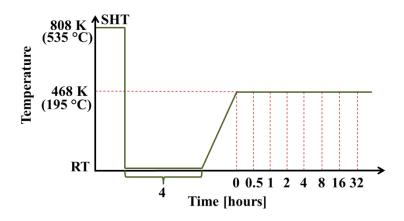
**Fig. 1** Heat treatment overview. After quenching from solution temperature (535 °C), samples were held at RT for four hours before heated to the 195 °C artificial ageing temperature (at a rate 26 °C/hour). Vertical dotted lines indicate ageing times where water-quenching to RT completed the ageing.
