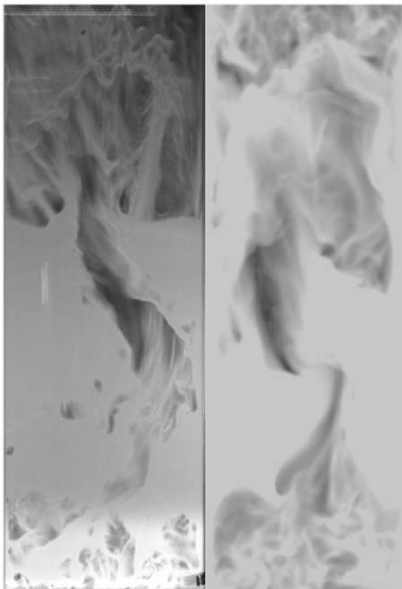
Figure 16: Visual comparison of the bed dynamics for the experiment (left) and the 3D simulation with adjusted grey levels and brightness (right) for case 7. The same images were used as in Figure 14. The animation comparing to experiments (Experimental_comparison.mpg) was made in this manner.
