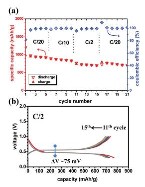
Fig. 4 (a) Rate capability tests of the 75MgH $_2\cdot$ 25CoO-based anode using LiBH $_4$  SE toward Li (different C-rates, 120 °C). (b) Display of the galvanostatic discharge–charge profiles from 11th to 15th cycle (C/2 rate).
