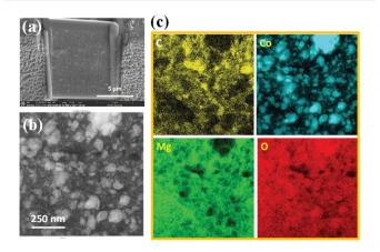
Fig. 5 STEM images of the as-assembled 75MgH $_2$ ·25CoO-based cell before cycling: (a) cross-section of the electrode side during thinning with FIB, (b) HAADF STEM image and the corresponding (c) EDS mapping.
