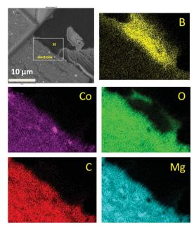
Fig. 6 Electron micrographs (FIB-SEM) of 75MgH<sub>2</sub>·25CoO-based cell after 2 cycles at the electrode/electrolyte interface and the corresponding EDS mapping of the selected area.
