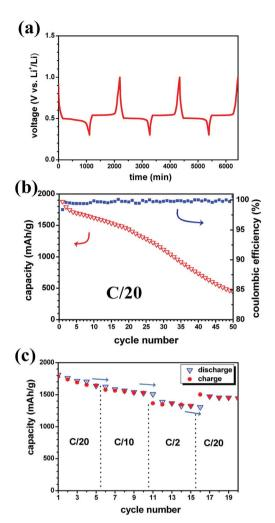
Fig. 2 (a) Display of the notable cyclability (voltage vs. time) of MgH $_2$  single anode using LiBH $_4$  SE toward Li (C-rate C/20, 120 °C). (b) Cycling performance as function of cycle number with the corresponding coulombic efficiency. (c) Rate capability tests of the same electrode.
