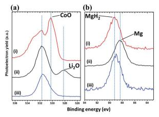
Fig. 7 (a) O 1s and (b) Mg 2s photoelectrons spectra regions of (i) the starting CoO/MgH $_2$  powders, (ii) discharged 75MgH $_2$ ·25CoO-based cell at 0.3 V and (iii) charged at 1 V.
