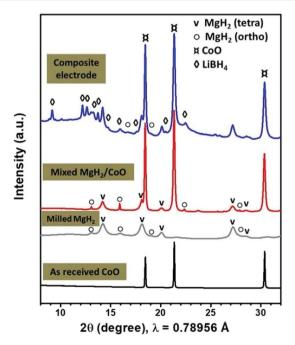
Fig. 1 SR-PXD patterns of the as-received CoO, 24 h milled MgH $_2$  and mixed MgH $_2$ /CoO, and after addition of the LiBH $_4$  solid electrolyte and C $_{\text{SP}}$  carbon black.
