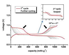
Fig. 3 Discharge–charge galvanostatic profiles of the  $75 \text{MgH}_2 \cdot 25 \text{CoO-based}$  anode using LiBH<sub>4</sub> SE toward Li (0.05C rate, 120 °C). Inset: looped discharge/charge curve for clarity.
