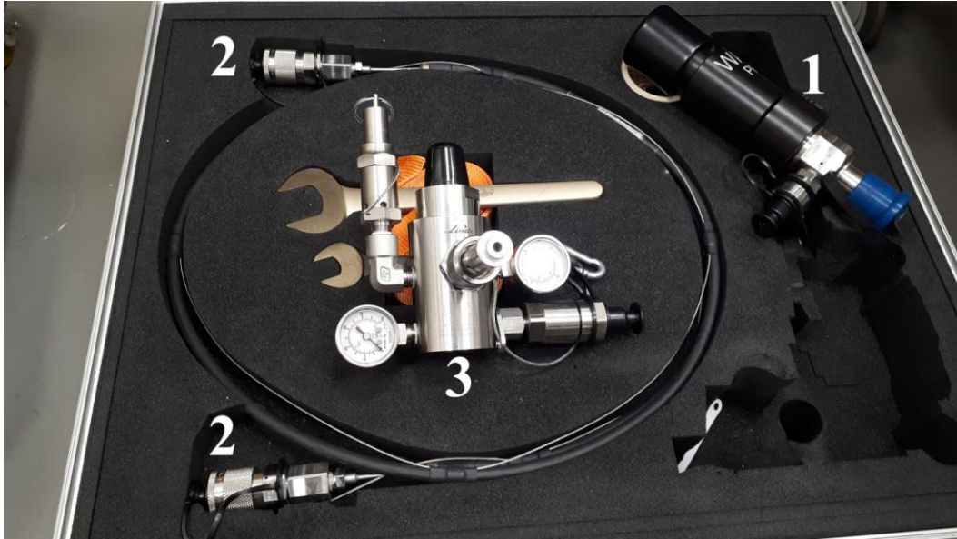
Figure 3. Linde H2 Qualitizer kit with numbered 1: Sample taking adapter “HG-004 adapter”; numbered 2: High pressure hose including 2 DN4 quick coupling from Walther and numbered 3: Pressure reducer for filling the sample taking container.
