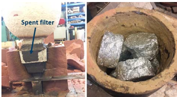
Figure 3 The cross section of the sand mould after test (left) and pressed Al kitchen foil for melting (right)
