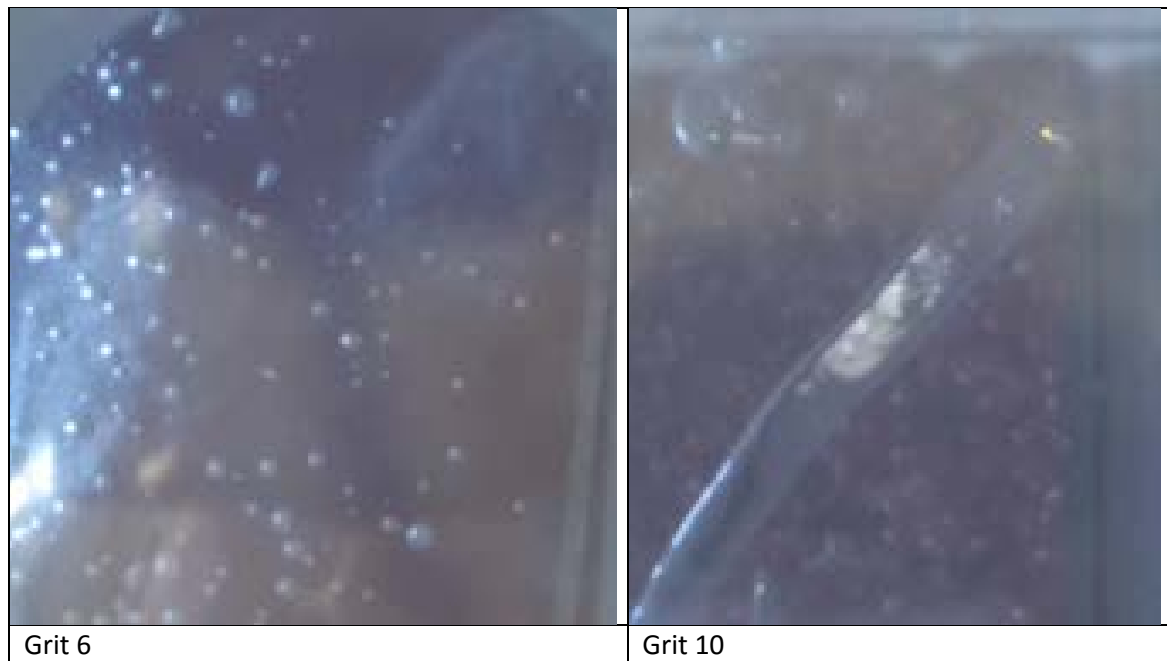
Figure 6: Priming of the filters taken through the glass showing good and bad priming of grit 6 and 10, respectively.
