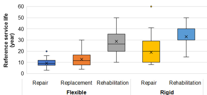
Fig. 6. Meta-analysis of the reference service life for the repair, replacement and refurbishment of flexible pavement.
