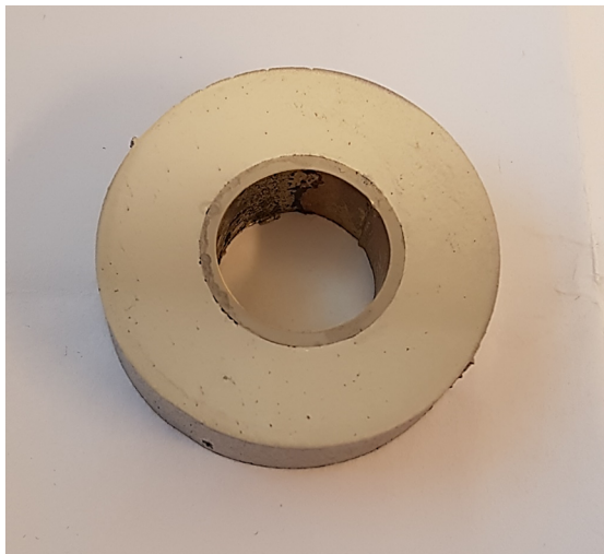
Figure 6: Image of a casting sample with a brass-coated steel pipe. Small cavities can be observed throughout the aluminum-steel interface.
