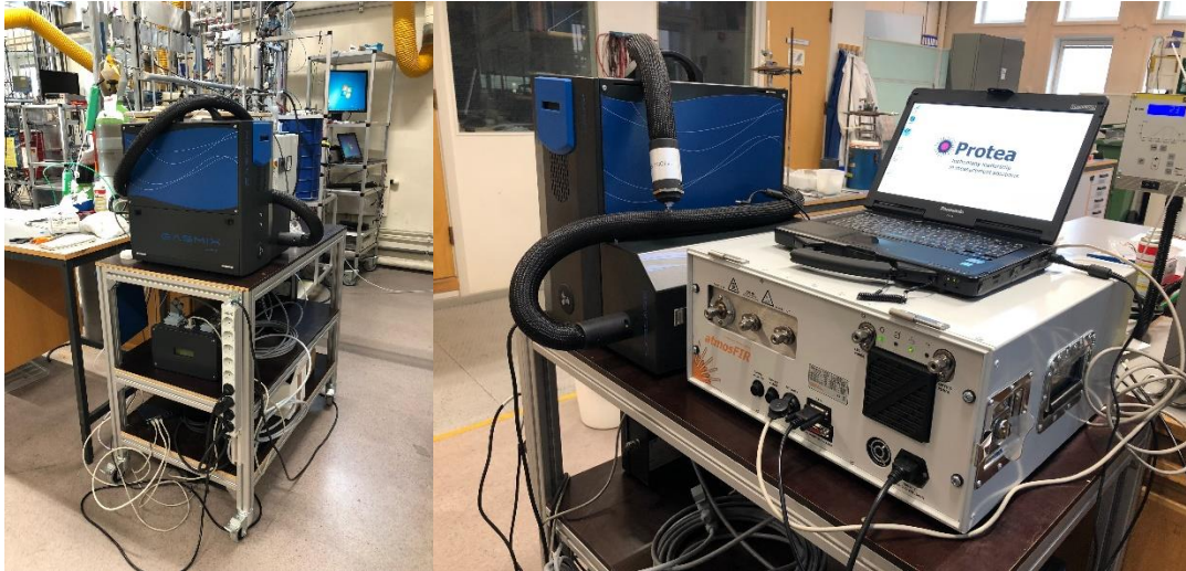
Figure 2. Experimental setup with Alytech gas mixer (left), Protea FTIR (right) and NEO Q CF 4 laser (below).
