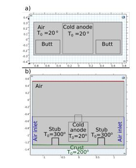
Fig. 1 Schematic of concept for anode pre-heating utilizing butts (a) and off-gas within the superstructure (b) along with initial conditions for temperature. The outer boundary conditions for (a) were set to adiabatic or convective in two separate cases in order to estimate the effect of insulation, while the boundary conditions for (b) were as specified.
