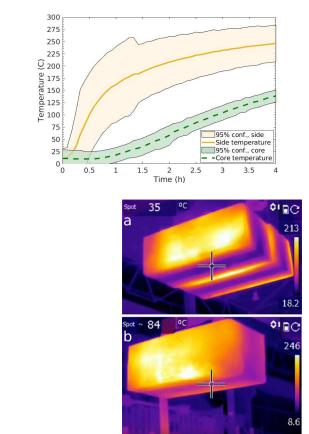
Fig. 5 Temperature evolution on side (solid orange) and core (dashed green) of anode for all pre-heating experiments with 95% confidence interval.
