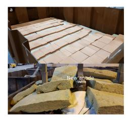
Fig. 3 Setup of insulation and bricks in anode container (a) and placement of butts and new anodes with insulating cover (b).
