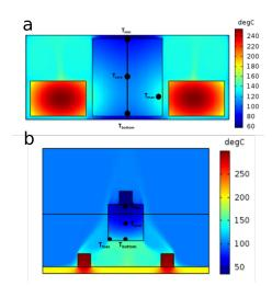
Fig. 2 Position of temperature sampling points and temperature distribution for pre-heating by butts (a) and within cell (b).
