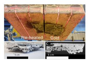
eration (a) with sample from cold anode (b) and CT image of the same sample (c).
