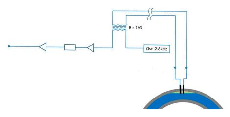
**Figure 7.** Principle of operation for conductivity measurement. Lower density displaced fluid (yellow) stratified above higher density displacing fluid (blue).
