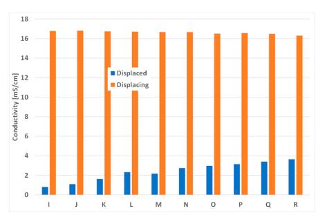
**Figure 9.** Fluid conductivity measured during 10 consecutive displacement experiments using the conductivity probe C0.
