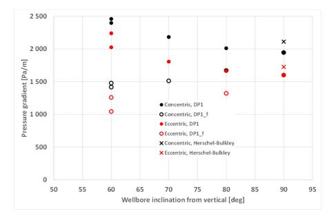
**Figure 16.** Measured pressure gradients DP1 for horizontal and inclined wellbore from experiments without inner pipe rotation, and corresponding frictional pressure gradients DP1\_f, assuming a fluid density difference of 100 kg/m3. Crosses show corresponding calculations using the values from Table 5.
