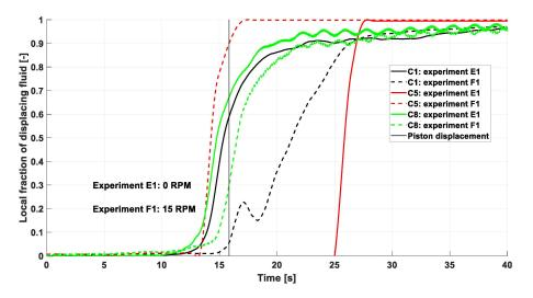
**Figure 17.** Effect of inner pipe rotation on displacement in inclined wellbore (60 degrees from vertical) with eccentric annulus (e = -0.42). Curves showing fraction of displacing fluid at station C (near inlet to washout section) without inner pipe rotation (experiment E1) and with inner pipe rotation (experiment F1). Azimuthal positions of probes (1, 5 and 8) are as shown in Figure 6.
