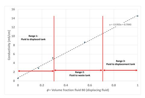
**Figure 8.** Measured conductivity (points) versus volume fraction of fluid B0. Stippled line shows the linear regression of the measurement points.
