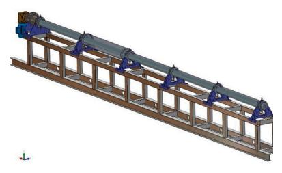
**Figure 1.** Test section with inlet to the right and outlet to the left. A torque motor for the rotating inner pipe is mounted at the outlet.
