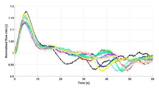
**Figure 10.** Normalized fluid flow rate versus time from start of displacement for the experiments with the automatic pump control.
