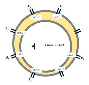
**Figure 6.** Schematic cross section of test section showing position of conductivity probes and inner pipe in eccentric position. Pressure ports (not shown) were located between probes 6 and 7.
