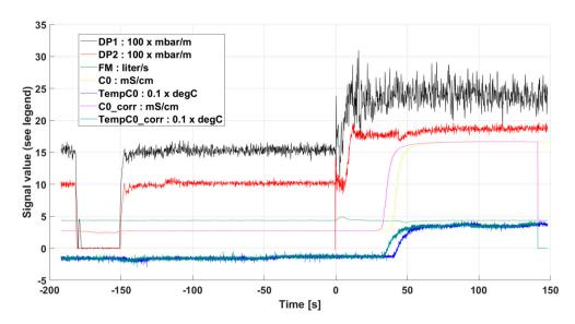
**Figure 14.** Experiment in concentric annulus with 60 degrees well inclination. Time traces of pressure gradients (DP1: black, DP2: red), flow rate (FM: green), conductivity of mixed fluid downstream of test section (C0: yellow), and temperature of mixed fluid downstream of test section (T0: blue).
