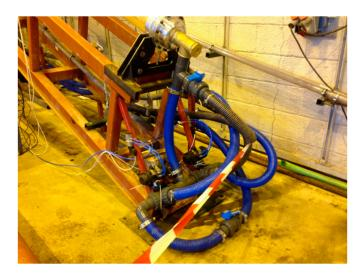
**Figure 5.** Piping and valves at inlet to test section. The valves V1 and V2 of Figure 2 were controlled from the PC using pneumatic actuators. A drain valve (blue handle) with corresponding hose (not shown in Figure 2) was used to drain the test section after an experiment.
