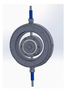
Figure 4. Bearing joint connecting two sections of inner pipe.
