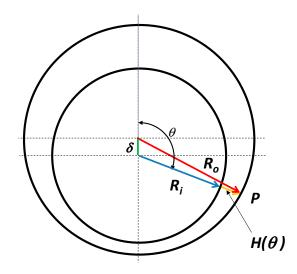
**Figure 13.** Definition of azimuthal angle  $\theta$  and angle-dependent gap  $H(\theta)$  for eccentric annulus.
