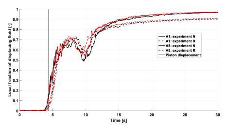
**Figure 11.** Local fraction of displacing fluid near the inlet (station A) and near the top (positions 1 and 8) for an experiment with inclined (60 degrees) concentric annulus (experiment N), and a repetition experiment (R), both without rotation of inner pipe.
