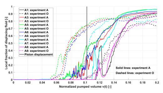
**Figure 12.** Displacement versus normalized pump volume for equivalent experiments in Experiments A and O. All measurements were conducted at Station A being 2 m from inlet.
