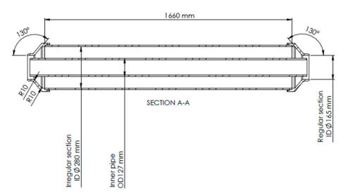
Figure 3. Details of the irregular section.
