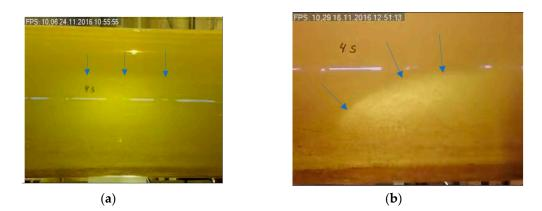
**Figure 18.** Displacement in washout section for horizontal flow in concentric annulus (**a**) and for eccentric annulus (**b**). Arrows indicate position of interface between displaced fluid and displacing fluid, where displacing fluid is below arrows (**a**) or below and to the right of arrows (**b**).
