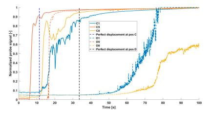
**Figure 19.** Measurement of displacing fluid fraction immediately upstream and downstream of the washout section for an experiment in horizontal wellbore with concentric inner pipe. Probes C1/D1 and C8/D8 measure fluid fraction near top upstream/downstream of washout section, while probes C5/D5 measure corresponding fluid fractions near the bottom.
