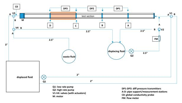
**Figure 2.** Process and instrumentation diagram for the flow rig. Note that probe C0 and valve V3 were positioned about 9.5 m downstream of the test section exit point.
