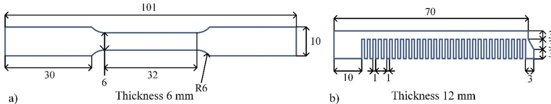
Figure 1 Dimensions of tensile specimens (a), and cantilever beams (b). All units in mm.
