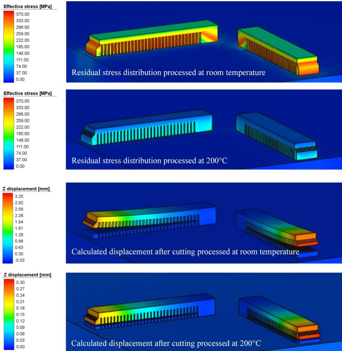
Figure 2 Residual stress distribution and calculated displacement after cutting for AlSi10Mg processed at room temperature and at 200°C
