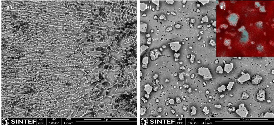
Figure 6 SEM images of a) as-built heat treatment condition - 0° specimen, b) T6 heat treatment condition - 0° specimen, c) EDS map of Al (red) and Si (cyan) of the T6 condition (same scale).
