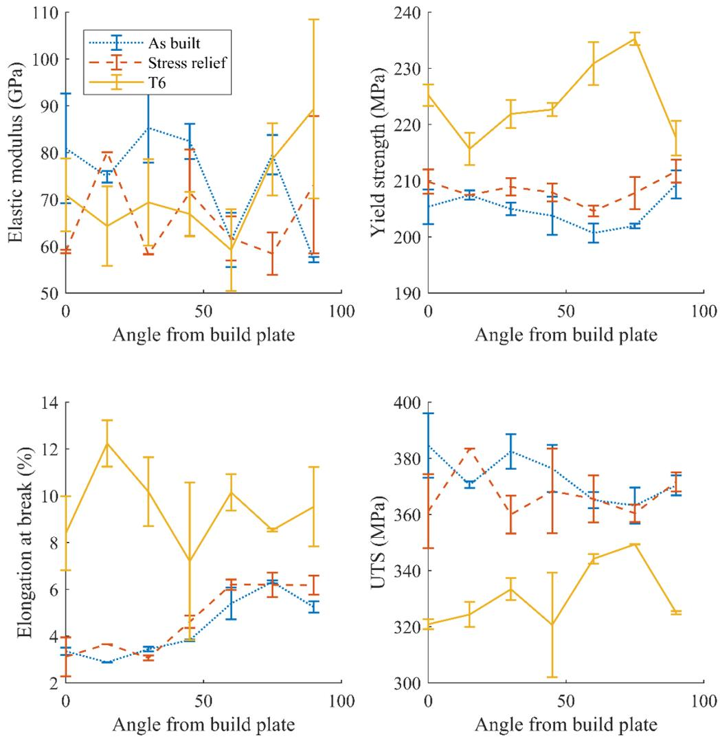
Figure 4 Tensile properties plotted as a function of specimen orientation with respect to the build platform
