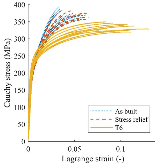
Figure 3 Cauchy stress plotted against the Lagrange strain for all 14 samples from each of the three heat treatment conditions
