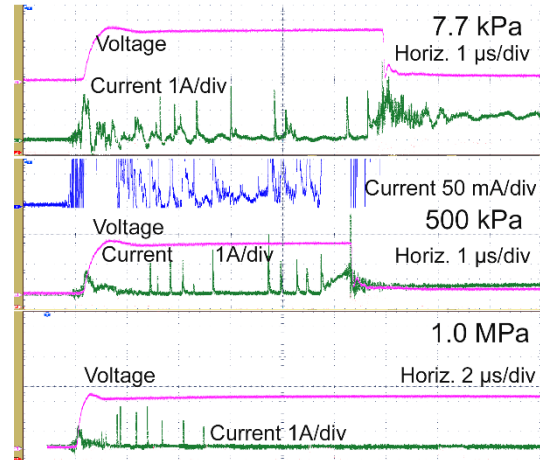
Figure 20. Reilluminations in negative 3 rd mode streamers at 356 kV. For the two streamers going to breakdown, there is 4 th mode the last approximately 0.5 \mu s.
