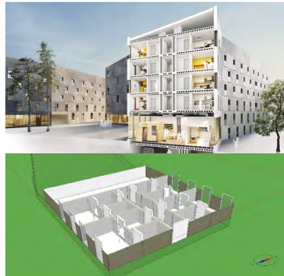
Figure 1: Computer generated view of the Testbed KTH building [source: property developer Einar Mattsson] and the building model generated in IDA-ICE.
