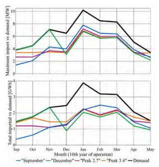
Figure 8: Four cases for peak heating reduction: (a) maximum peak values for Furuset's heating demand vs. imported district heat [MW], (b) overall heat demand of Furuset vs. imported heat from district heating [GWh]
