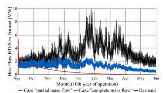
Figure 6: Comparison between Furuset's heat demand and the heat flow rate for the BTES, for nine months of BTES discharging, after ten years of operation
