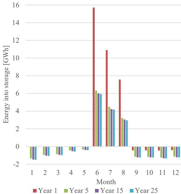
Figure 4: Estimated monthly heat for charging and discharging the BTES for several years of operation [Tvärne18]
