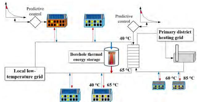
Figure 1: The planned micro energy system in Furuset
