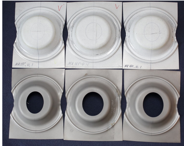
Figure 5: Marciniak-Kuczynski samples after the test
