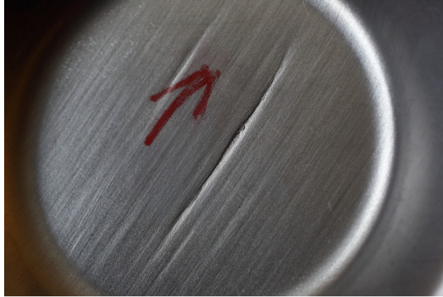
Figure 9: Roning and multiple local necks in an Marciniak-Kuczynski sample
