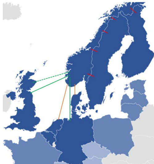
Figure 3 Norway and its electrical connections to other countries, AC (red), existing HVDC (orange), HVDC under construction (green), HVDC currently under consideration (green stippled).
