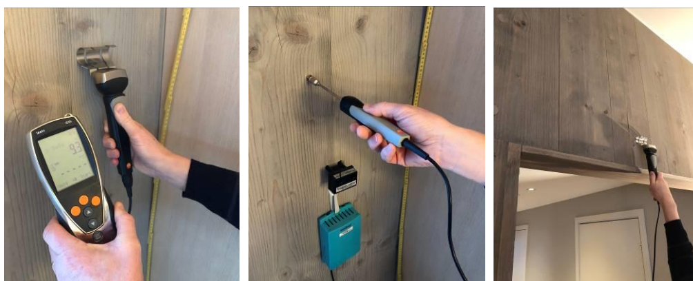
Fig. 4. Left: The non- destructive moisture meter on the inner surface of the exterior CLT wall element. Middle: The surface thermocouple on the inner surface of the exterior CLT wall element. Right: The non- destructive moisture meter on the surface of the interior CLT wall element.
