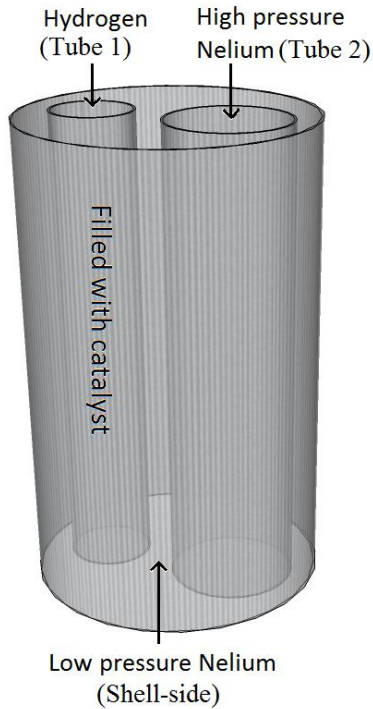
Figure 1: Illustration of the heat exchanger geometry.
