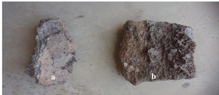
Figure 1. Refractory material (Fig 1 a) and slag (Fig 1 b) collected after shutdown of the combustion appliance.
