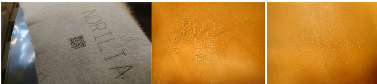
Fig. 7. To the left: Finished hide with markings, the middle and the right shows examples of hides with readable but deformed laser engravings after coming back from the tannery.
