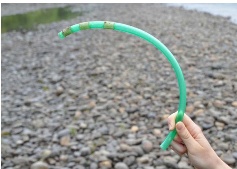
Figure 2.1: flexible rubber tube with attached rings indicating shelter depth
