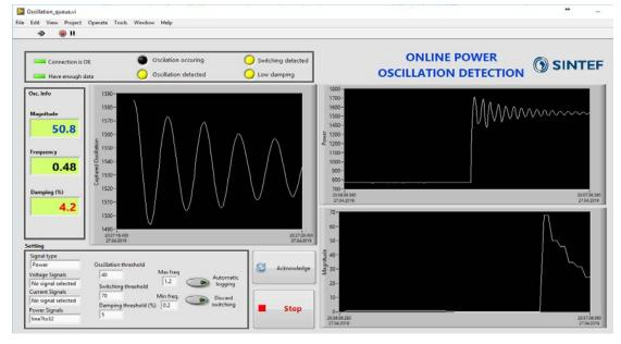
Figure 9. An oscillation captured by the online monitoring tool.
