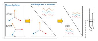
Figure 3. Conversion of phasors to waveforms to enable PHIL testing.
