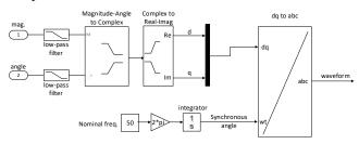
Figure 4. Implementation of phasor-to-waveform conversion.
