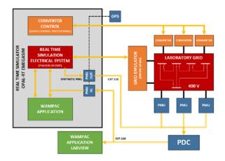
Figure 2. Overview of the testing platform.
