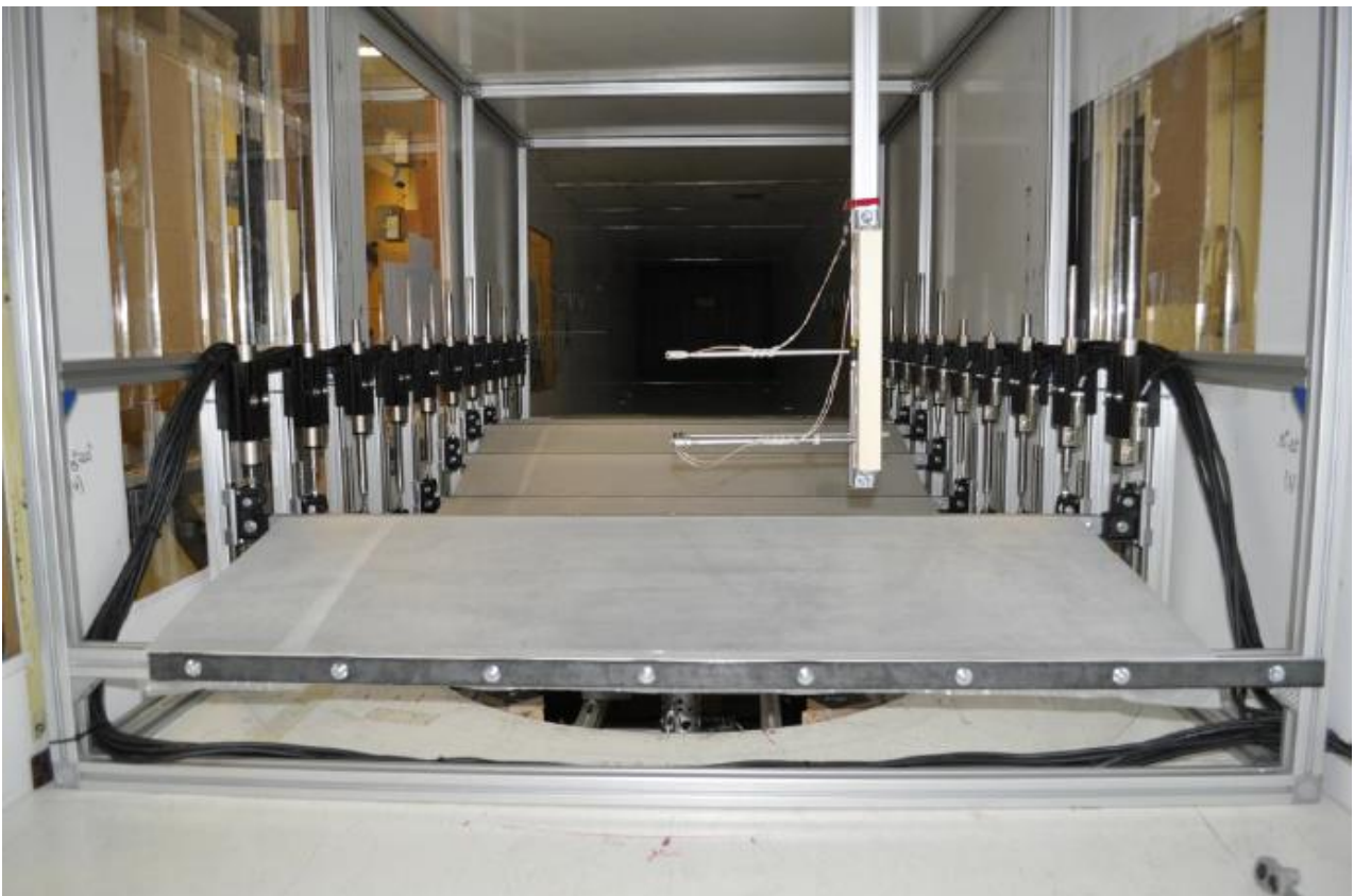
Figure 14 Model set-up for the wave influence experiment with a travelling wave floor in the wind tunnel. In the middle of the photograph, the bridge section model (1:40) can be seen [16].
