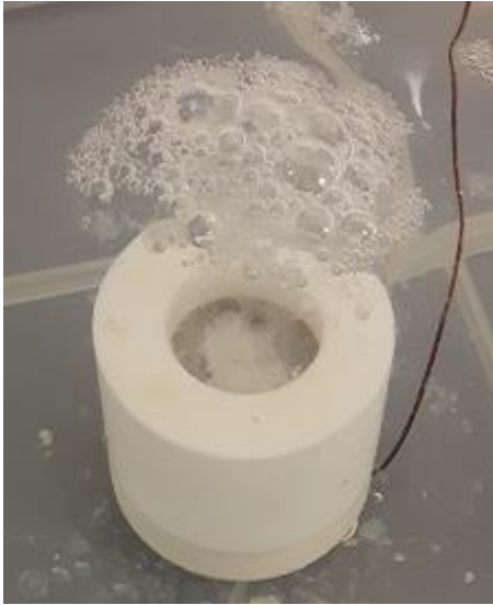
Fig. 8: Gas evolution on aluminium specimen at 60 Hz.
