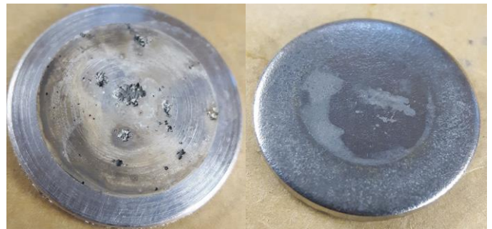
Fig. 7: Aluminum (left) and steel (right) specimens after corrosion test and cleaning process.
