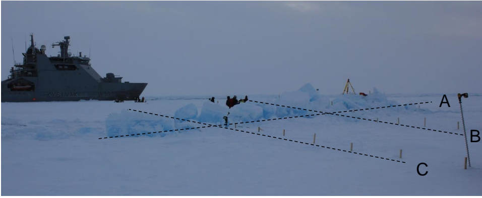
Figure 5 Photo of the ridge R2-2012 and illustrates the lines established for drilling of holes along the spine A and cross sections B and C.
