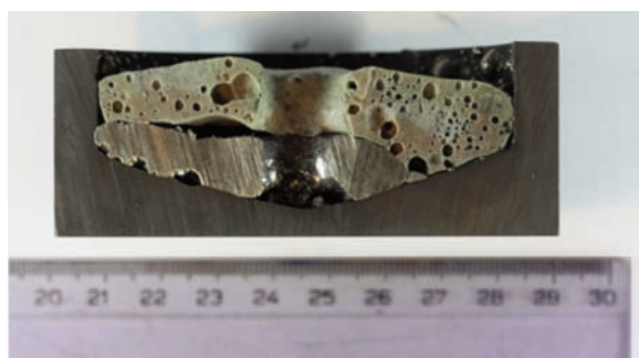
Figure 3. Cross section of the crucible after the smelting test.
