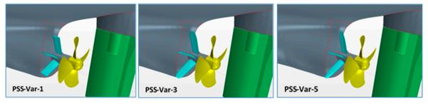
Figure 7. Evolution of PSS design in the process of design exploration.
