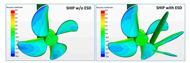
**Figure 15.** Cavitation domains on the propeller and ESD. (PSS-Var-5, full scale, Vs = 16 kn, ballast draught).
