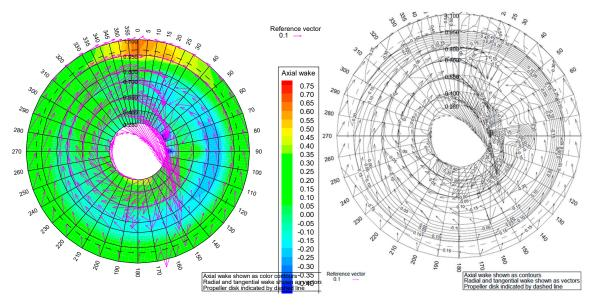
**Figure 21.** 3D wake measurements at a plane midway between the propeller and rudder, with a working propeller, without PSS, at 14 kn.
