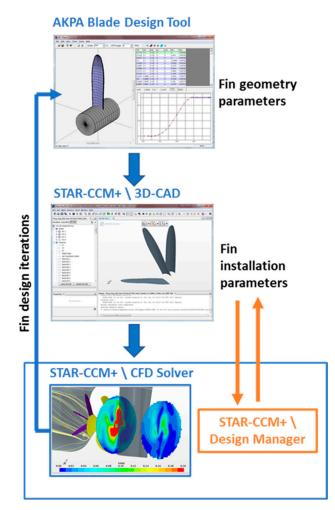
Figure 6. Overall flow chart of the ESD design workflow.
