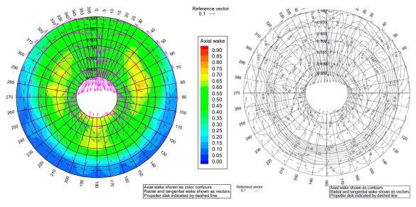
Figure 19. 3D wake measurements at the propeller plane, without PSS, at 14 kn.
