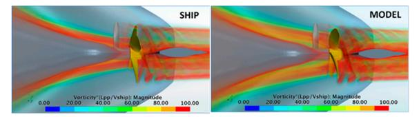
**Figure 26.** Vorticity field in the ship wake around ESD and propeller location on a full scale and a model scale. (Vs = 14 kn).
