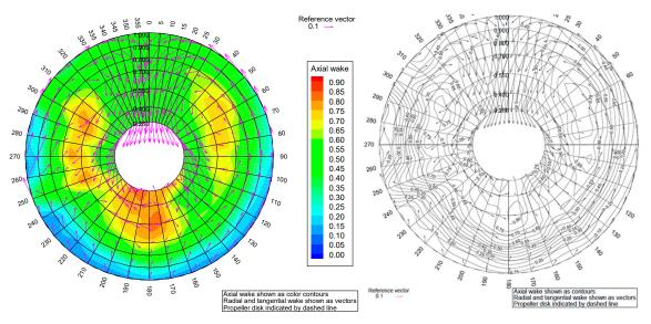
Figure 20. 3D wake measurements at the propeller plane, with PSS, at 14 kn.
