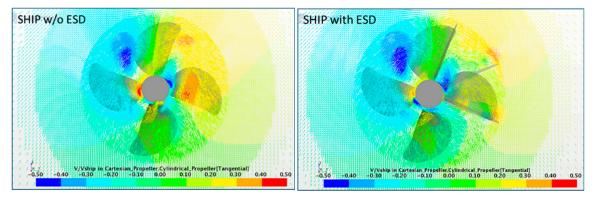
**Figure 8.** Distribution of the tangential velocity on section "Sect 1" in front of the propeller, seen from upstream (PSS-Var-5, full scale, Vs = 14 kn).
