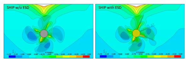
**Figure 9.** Distribution of the axial velocity on section "Sect 1" in front of the propeller, seen from upstream (PSS-Var-5, full scale, Vs = 14 kn).
