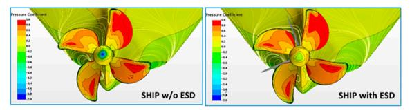
**Figure 13.** Pressure distribution on the hub and pressure side of propeller blades (PSS-Var-5, full scale, Vs = 14 kn).
