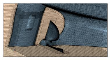
Figure 1. Fragment of computation mesh in the vessel stern region.
