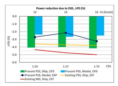
Figure 25. Comparison of power savings due to ESD installation.
