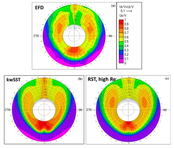
**Figure 4.** Measured and computed nominal wake field around the ESD location. (Model scale, Vs = 14 kn, without ESD). (**a**) measured results. (**b**) CFD results using kwSST. (**c**) CFD results using RST, high Re.
