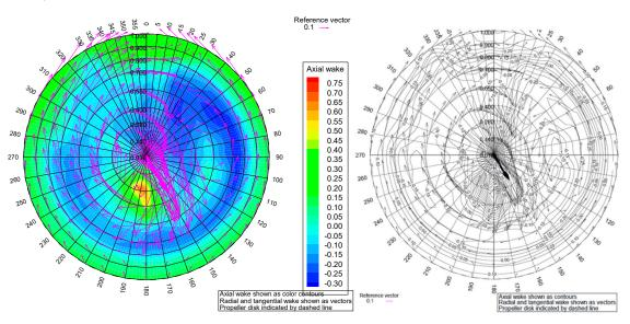
**Figure 24.** 3D wake measurements at a rudder stock plane (AP), with a working propeller, with PSS, at 14 kn.
