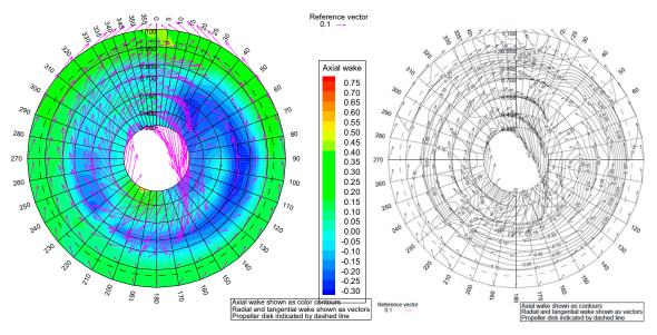
**Figure 23.** 3D wake measurements at a rudder stock plane (AP), with a working propeller, without PSS, at 14 kn.
