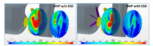
**Figure 10.** Distribution of the kinetic energy of transverse flow on sections "Sect 2" and "Sect 3" downstream of the propeller (PSS-Var-5, full scale, Vs = 14 kn).
