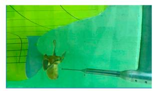
Figure 16. 3D wake measurements setup.
