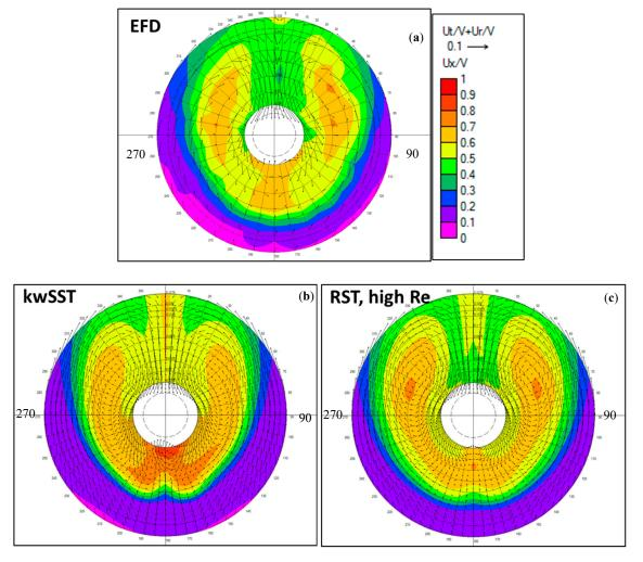
**Figure 3.** Measured and computed nominal wake field on the propeller plane. (Model scale, Vs = 14 kn, without ESD). (**a**) measured results. (**b**) CFD results using kwSST. (**c**) CFD results using RST, high Re.
