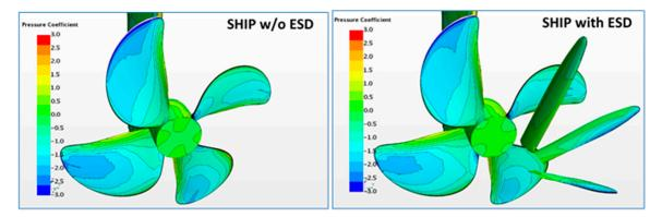
Figure 14. Cavitation domains on propeller and ESD. (PSS-Var-5, full scale, Vs = 14 kn, ballast draught).
