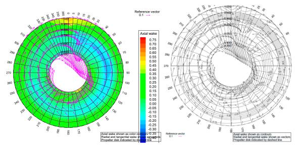
**Figure 22.** 3D wake measurements at a plane midway between the propeller and rudder, with a working propeller, with PSS, at 14 kn.
