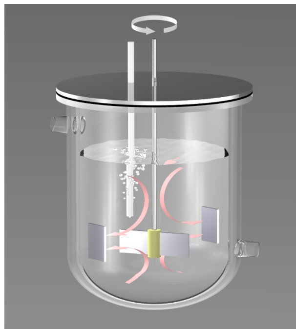
Figure 8. Sketch of the reactor with specimens placed as both impeller blades and stationary
