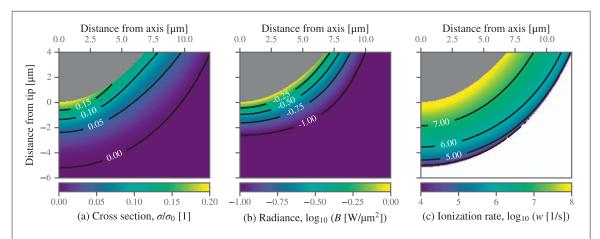
**Figure 3.** Streamer head (in grey) with  $r_p = 6 \mu m$  and  $V_0 = 100 \text{ kV}$ , placed d = 10 mm from the planar electrode. The cross section (a), radiance (b), and photoionization rate (c) are calculated by (7), (2), and (5), respectively, applying the parameter values stated in the first paragraph of section 4. The *y*-axis is equal for all the plots.
