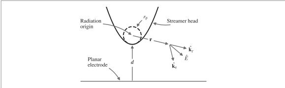
Figure 2. Sketch of a hyperbolic streamer head and relevant variables.
