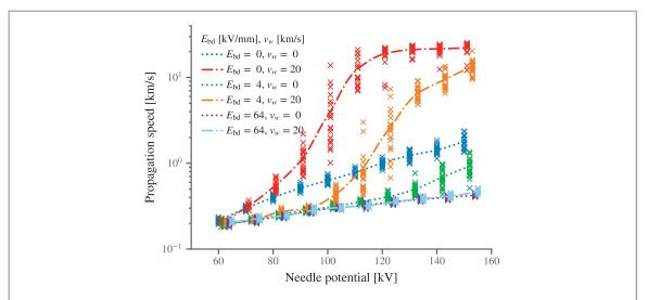
**Figure 7.** Average propagation speed for the middle of the gap (z between 2.5 mm and 7.5 mm). The onset of the fast mode is delayed when the field within the streamer channel is increased. Each marker is a simulation (20 for each voltage, 1200 in total) and the lines are interpolated to the average.  $v_w = 0 \,\mathrm{km} \,\mathrm{s}^{-1}$  implies no added speed from photoionization.
