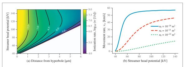
**Figure 4.** (a) Ionization rate w along z-axis for different  $V_0$ . 100 kV corresponds to figure 3(c). (b) Maximum movement rate  $v_w$  calculated by (8) assuming p=0.001. The transition is sharpest for  $\sigma_0=10^{-20}$  m $^2$  followed by  $10^{-21}$  m $^2$ , while  $10^{-22}$  m $^2$  resembles a linear increase. The magnitude is linearly dependent on  $B_0$  and inversely dependent on p.
