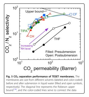
included in Fig. 4c, d, and indicate that gas humidification, as well as film submersion (especially at high RH), benefits membrane separation efficacy. Except for THF-cast specimens (which are the least selective before and after submersion), the highest selectivity values for presubmersion membranes range from 46 to 53, whereas those for postsubmersion membranes vary from 57 to 61 at  $\approx$ 90% RH.
