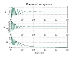
Figure 10: Simulation results from regulated and distributed mass-damper-spring system with nonlinear spring stiffness. Green graph denotes local solution and blue graph denotes global solution
