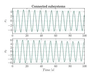
Figure 7: Simulation result of speed regulated mass-damperspring system implemented in a distributed system. Green graph denotes local solution and blue graph denotes global solution.
