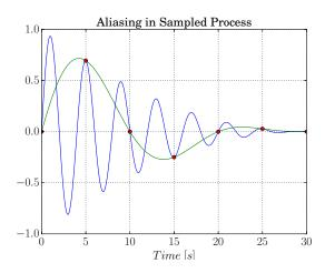
Figure 4: Aliasing in sampled system. The blue graph represents the process to be sampled, the read dots are the sampled values and the green graph is the recreated process from the sampled data.
