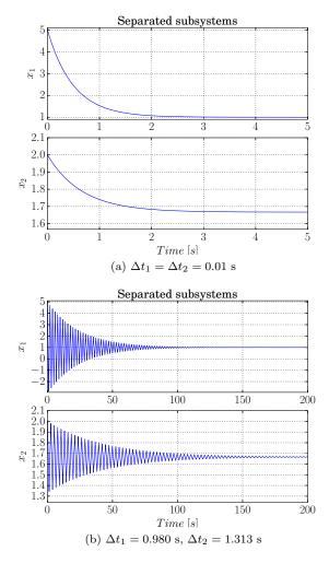
Figure 2: Simulation results of separated subsystems with different time steps.
