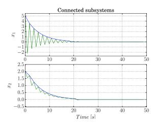
Figure 6: Simulation result of two subsystems with stable local solvers connected as in a distributed system. Green graph denotes local solution and blue graph denotes global solution.
