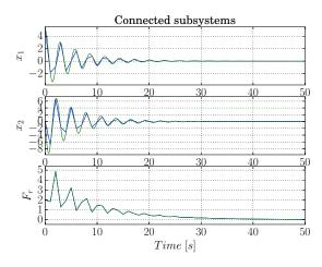
Figure 9: Simulation results showing the speed controlled mass-damper-spring system. Green graph denotes local solution and blue graph denotes global solution.
