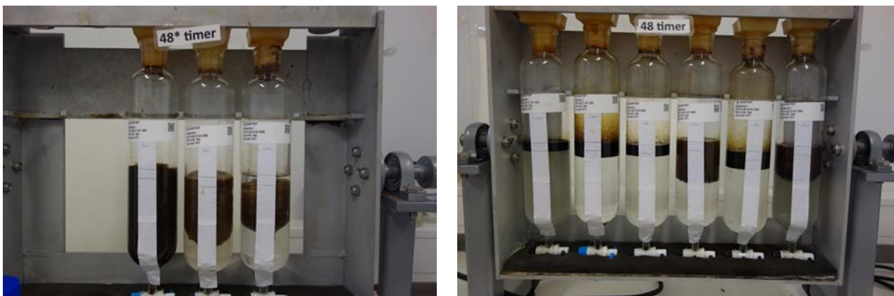
Figure 3-4: Stability of Oda emulsions of 150, 200 and 250°C+ residues (left) and effect of emulsion breaker (right)
