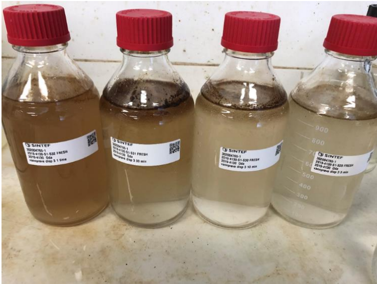
Figure 4-11: Water samples from 3. Round of dispersant application. From Left to Right: 60, 30, 10 and 3 min. after third application.
