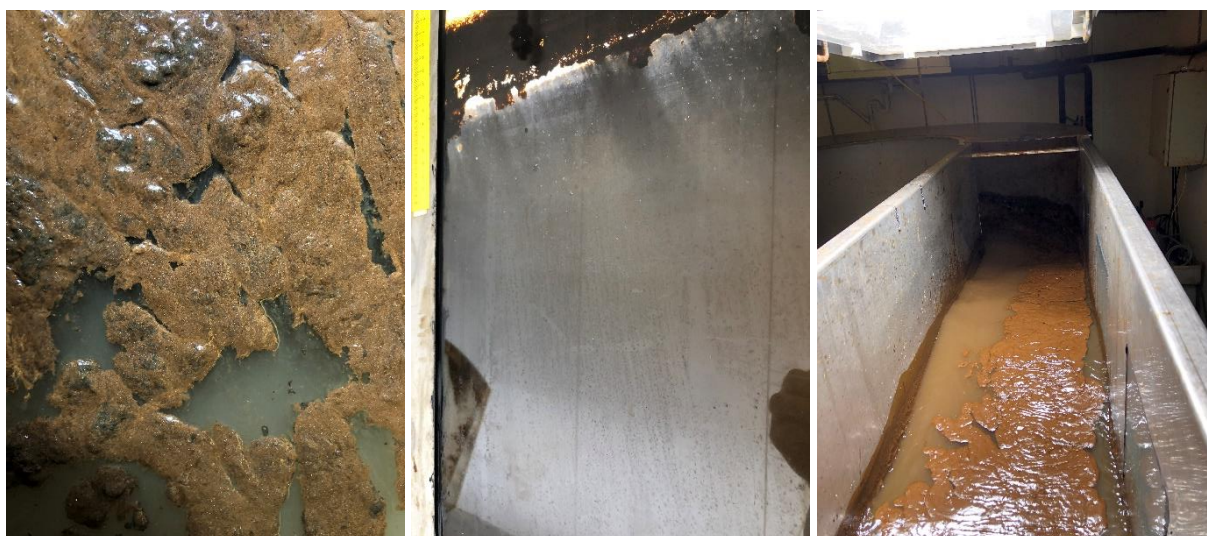
Figure 4-10: Left: The 3. application once again breaks the emulsion. Middle: More dispersed oil observed in the water phase (3 min. after application). Right: Surface oil (emulsion) 60 minutes after the third application – the colour of the water indicates that more oil is even more dispersed (visc. 6015 mPa.s, water content 32 vol.%)
