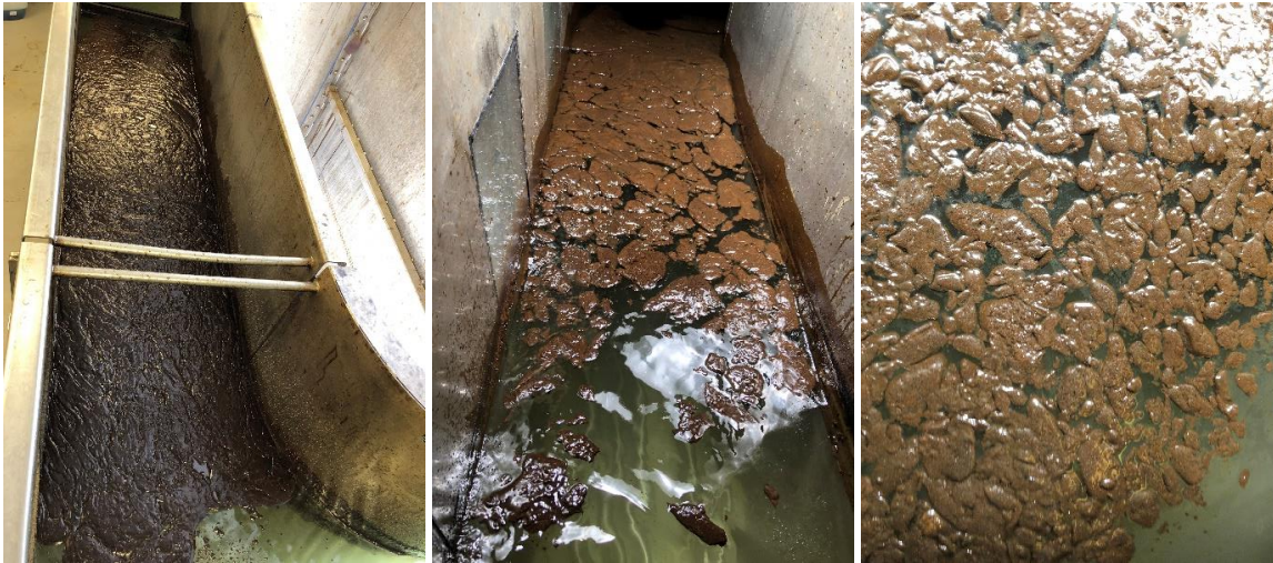
Figure 4-7 Left: The surface emulsion before application (visc. 13 860 mPa.s). Middle and Right: After 1. round of dispersant application, the structure of emulsion is broken to large patches. Viscosity reduced to 8900 mPa.s.
