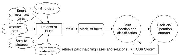
Figure 1: A proposed architecture for fault handling in distribution networks based on machine learning techniques.
