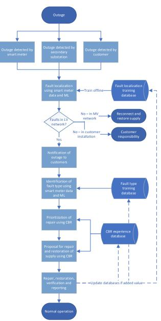
Figure 2: Flow chart for fault handling in low voltage distribution networks in 2030/2040 utilising ML
