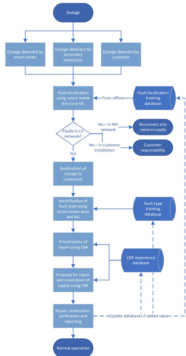
**Figure 2: Flow chart for fault handling in low voltage distribution networks in 2030/2040 utilising ML**
