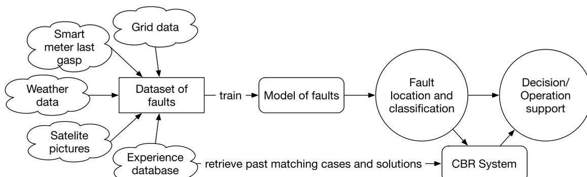
**Figure 1: A proposed architecture for fault handling in distribution networks based on machine learning techniques.**
