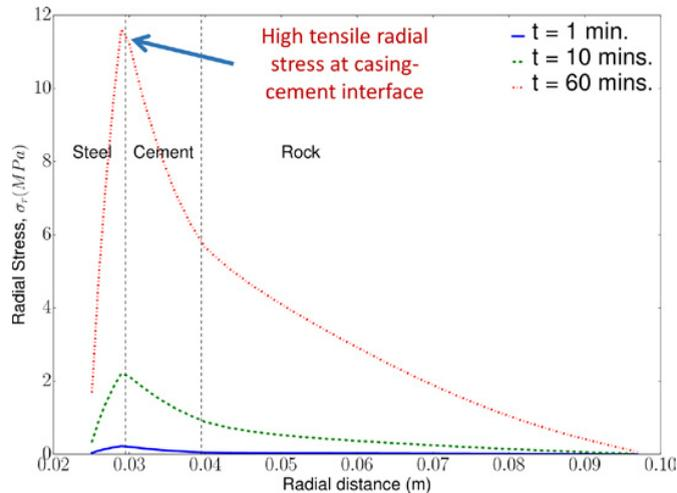
Fig. 6. Radial stress profiles as a function of radial distance for cooling at 1°C/min.
