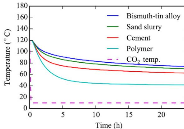
Fig. 8. Temperature at the casing/sealant interface as a function of time while injecting CO<sub>2</sub> at 10°C.
