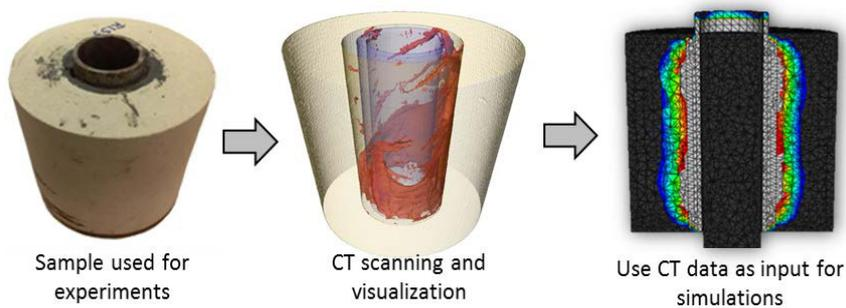
Fig. 7. An illustration of how samples used in experiments were first CT scanned, then reconstructed in 3D (including all defects), and finally used as input in numerical simulations of stress/stain effects.
