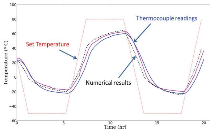
Fig. 4. Comparison of cement-casing interface temperature with top and bottom thermocouple readings.
