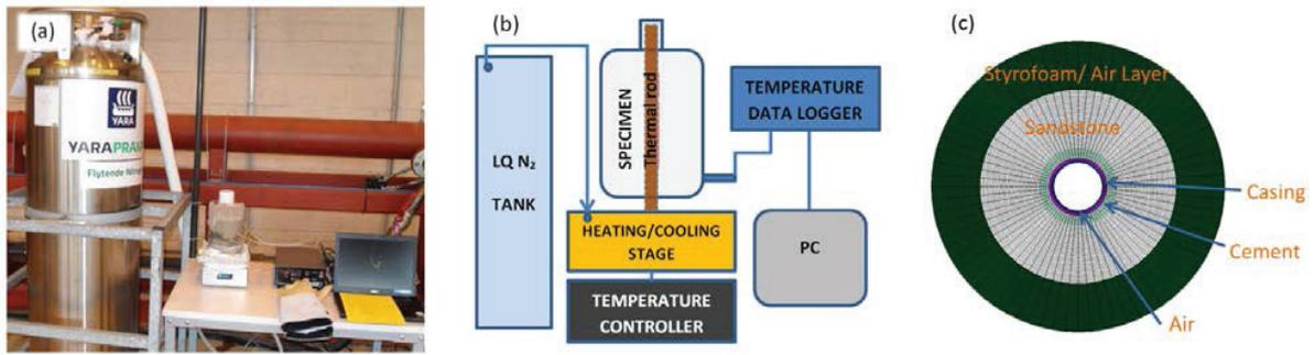
Fig. 1. (a) Picture of the thermal cycling set-up in the laboratory, (b) Schematic drawing of the constituents of the set-up, (c) Samples used for thermal cycling experiments as seen from above.
