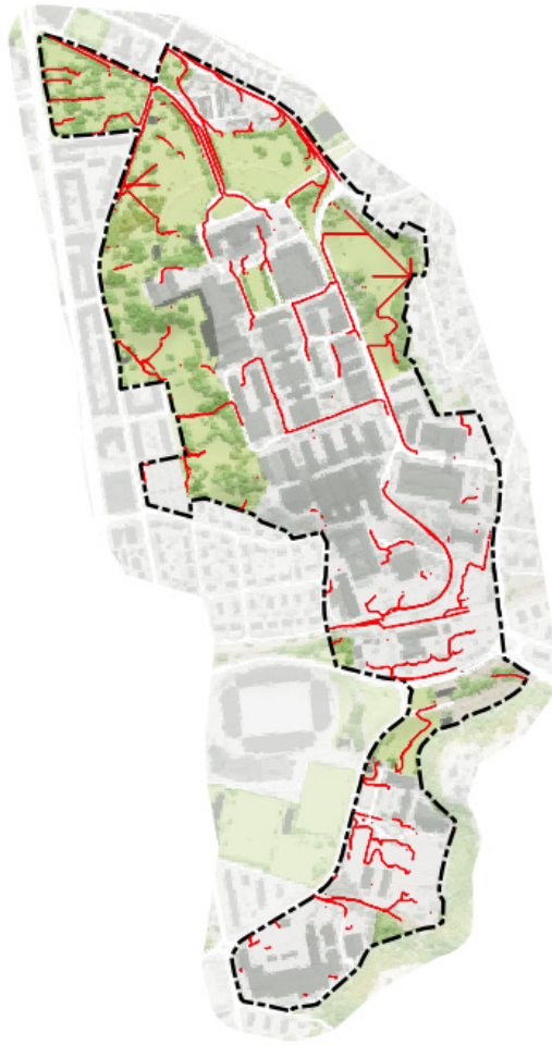
Figure 47: Example Output Vector "Main Flow Path Points" in red and a WMS background map.
