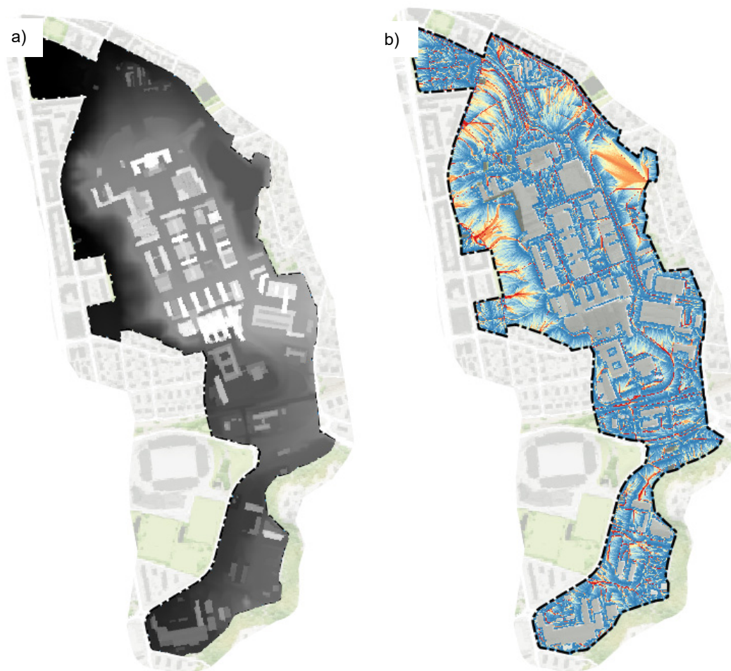
Figure 46: a) Example Input Raster "Combined Elevation Model" with data from the dtm for terrain and from dsm for buildings, also a WMS background map. b) Example Output Raster for flow accumulation, from low (blue) to high (red) accumulation and a WMS background map.
