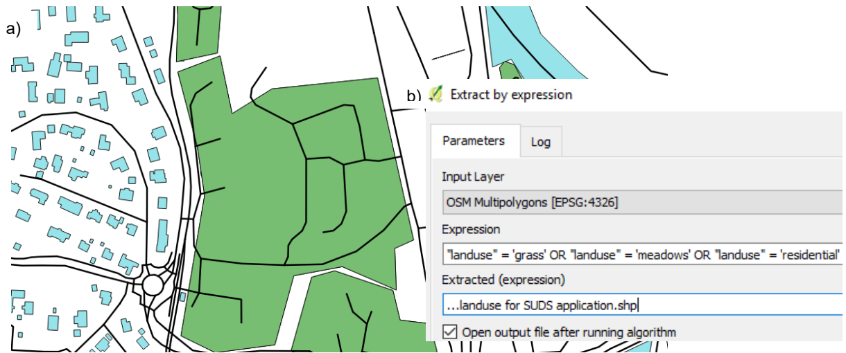
Figure 15: Example Open Street Map output, showing "Vector 1 – OSM lines", "Vector 2 – OSM multipolygons" and extracted "Vector 4 – OSM landuse" highlighted in green and b) appropriate working sheet for landuse extraction by [QGIS – Extract by expression].
