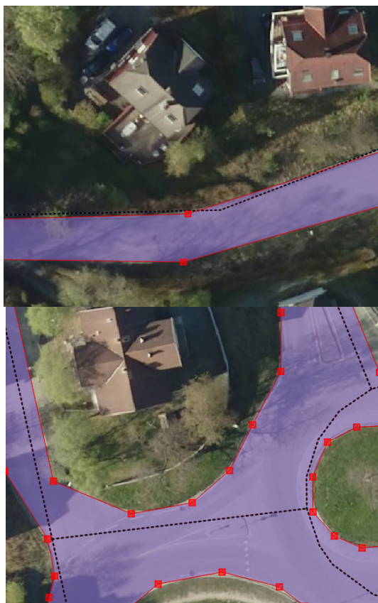
Figure 28 Example error correction for the OSM street vector, showing the dotted OSM street lines, selected buffer polygon and adapting nodes in lilac and a WMS orthophoto layer map in background, a) correction for off-centre OSM street line, b) correction for validation errors due to the buffer creation in a crossing section.
