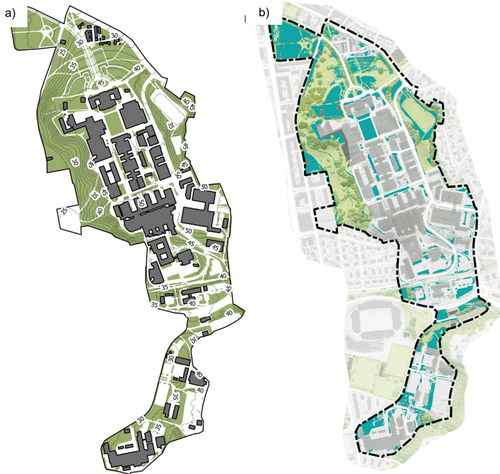
Figure 45: a) Example Input Vectors showing building polygons in black, landuse polygons which enable SUDS applicates in green and elevation lines (not needed in the model). b) Example Output Vector for "Potential SUDS Areas", highlighted in blue and a WMS background map.
