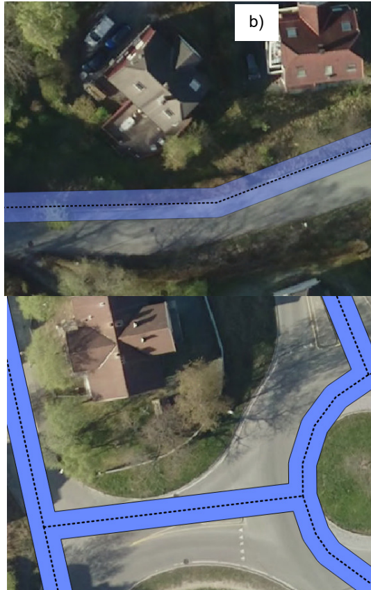
Figure 27: Example errors in the OSM street vector, showing the dotted OSM street lines, blue buffer polygon and a WMS orthophoto layer map in background, a) off-centre OSM street line, b) validation errors due to the buffer creation in a crossing section.
