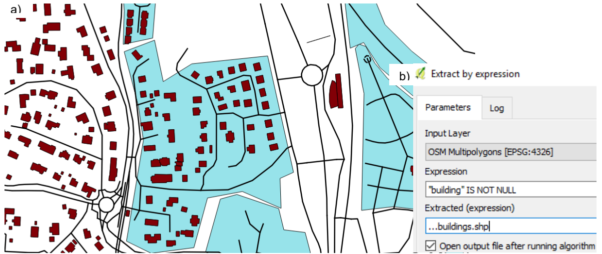
Figure 14: Example Open Street Map output, showing "Vector 1 – OSM lines", "Vector 2 – OSM multipolygons" and extracted "Vector 3 – OSM buildings" highlighted in red and b) appropriate working sheet for building extraction by [QGIS – Extract by expression].
