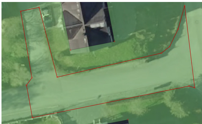
Figure 20 Example cut off via "Add ring" for the landuse vector correction, showing green landuse polygon, a WMS orthophoto layer map in background and the trace line in red, available if the cutting line doesn't touch the outline.
