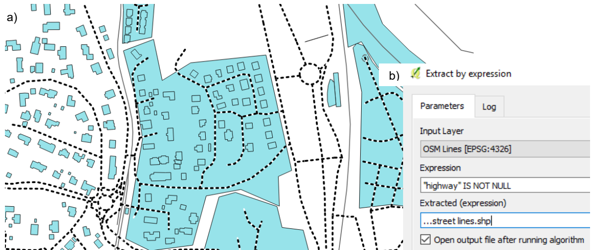
Figure 16: Example Open Street Map output, showing a) "Vector 1 – OSM lines", "Vector 2 – OSM multipolygons" and extracted " Vector 5 –street lines" highlighted via dotted lines and b) appropriate working sheet for street extraction by [QGIS – Extract by expression].
