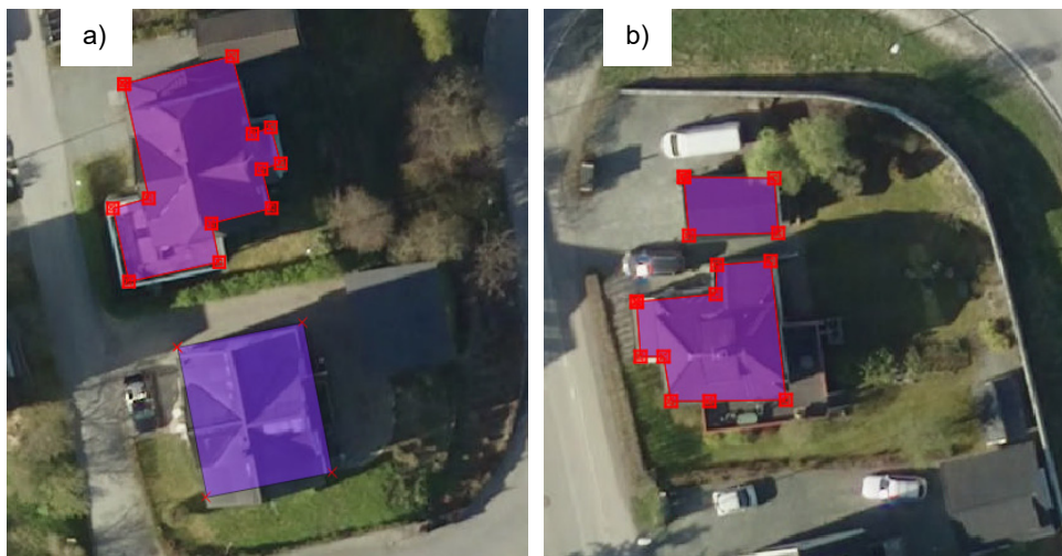
Figure 18 Example error correction for the OSM building vector, showing red building polygon and a WMS orthophoto layer map in background, a) correction for not complete drawn polygon, b) add missing polygons.
