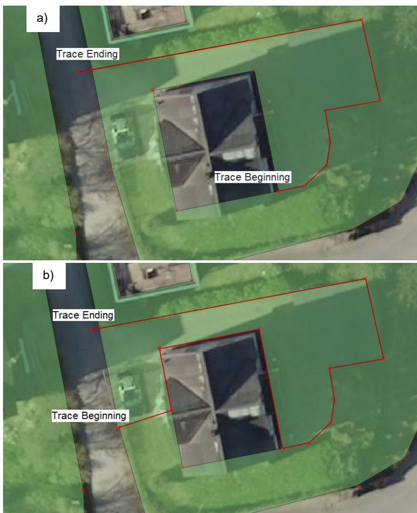
Figure 21 Example cut off via "Split feature" for the landuse vector correction, showing green landuse polygon, a WMS orthophoto layer map in background and the trace line in red, a) wrong tracing, the cutting line must cut off the polygon part completely, b) right tracing, if necessary follow an outline to cut off a complete part
