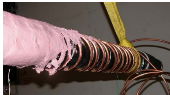
Figure 2. Embedding the copper pipes in a thermally well-conducting compound to provide a good temperature control of the cable surface.
