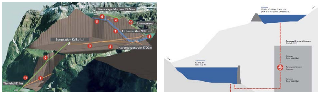
Figure 1. Cutaway graphics of the Limmern PSHP (source:[13]).
